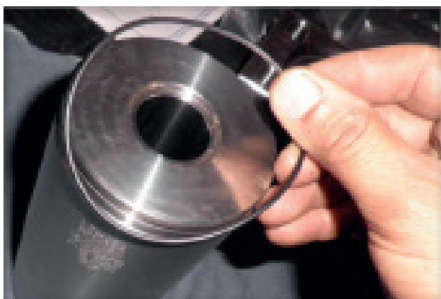
7° - Introduce the O-Ring into shell's recess.
