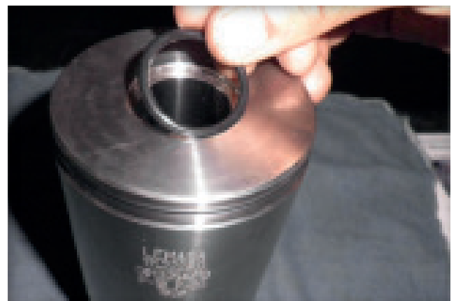
8° - Introduce the O-Ring into shell's groove.
