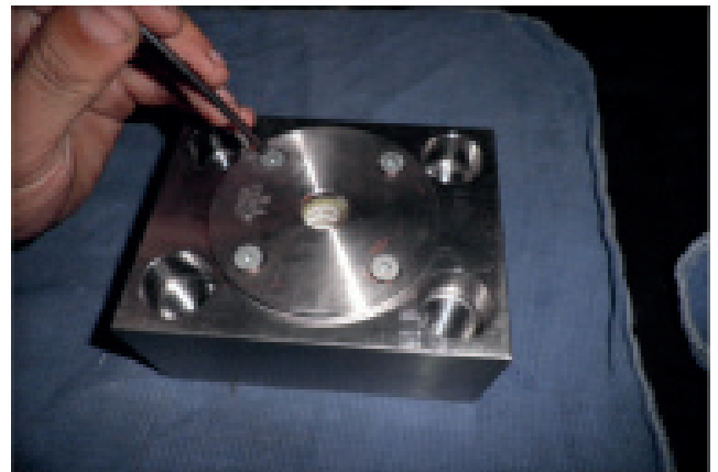
6° - Screw the Support Disk in "X".
