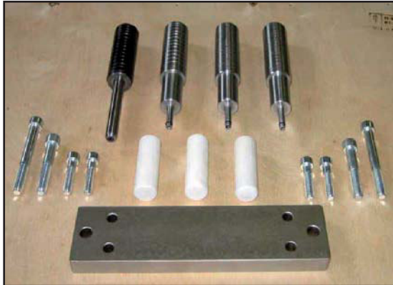
- ATR044. Tools for assembly/disassembly supplied with the pump.
